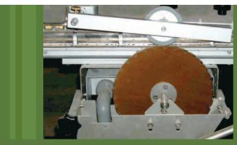
Selvedge gumming unit with reservoir for minimum glue application\*
