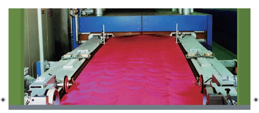
Short controlled fabric guidance for optimum feeding of even extremely delicate knitted fabrics. Uniform pinning by two driven draw rollers in the infeed unit.
