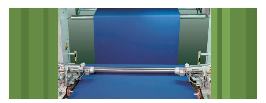
Delivery track lengths up to 4m. The delivery tracks are designed to accommodate all the auxiliary equipment necessary for the treatment of knitted and woven fabrics. The delivery unit can contain not only the standard tension roller (control range -10% to +35%) but also other equipment such as:
