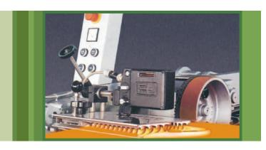
Mechanical scroll spindles, either two, three or four on each side
