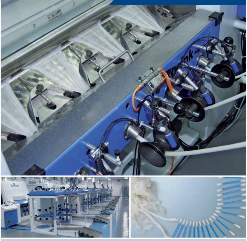
Optimal and gentle fibre opening. Very high sliver evenness. Simultaneous deposit of 4 slivers into 4 cans.
