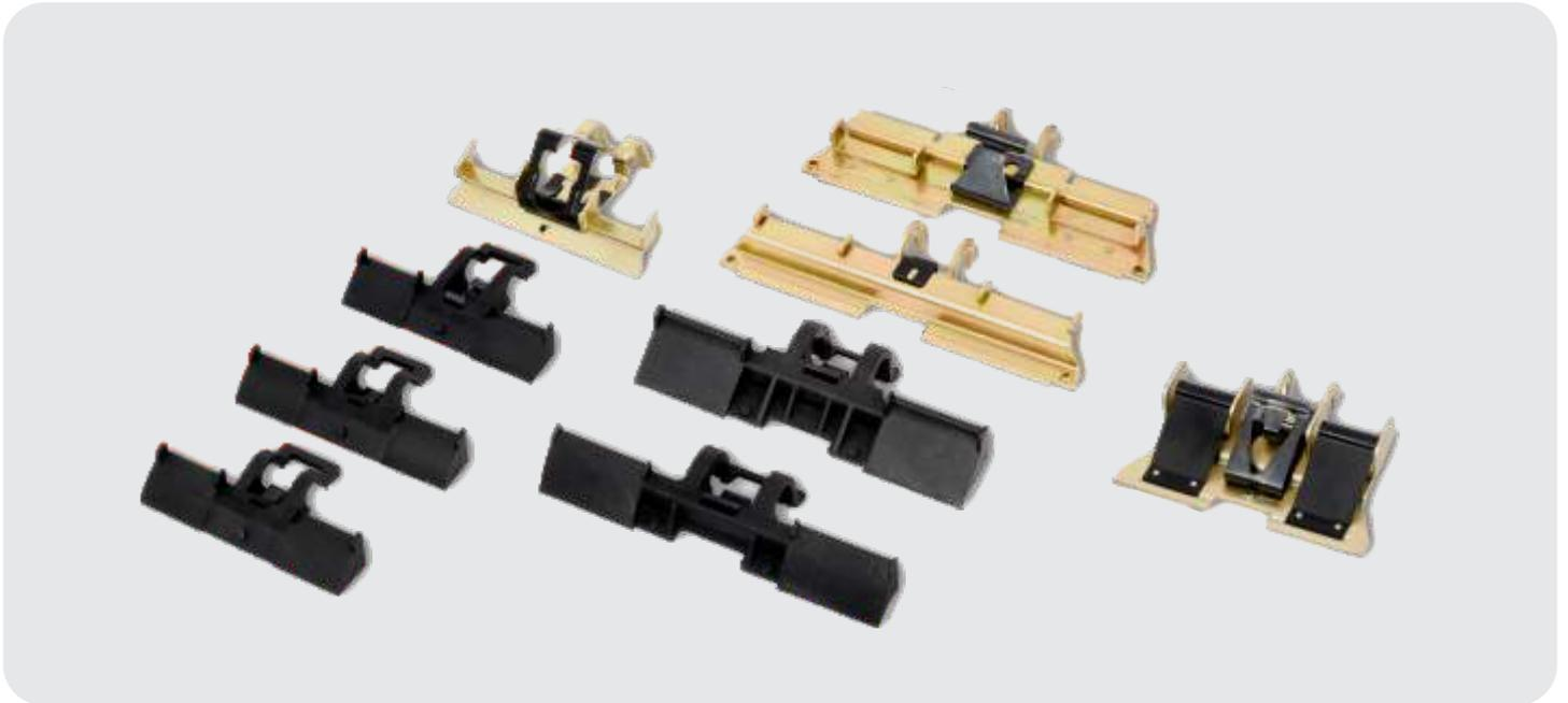
**C**radles discharge the important function of keeping the apron in position over the rotating apron top roller so that fibres are effectively guided in the main draft zone. TeraSpin cradles are made with Fibre Reinforced Plastic (FRP) for long life and ease of handling.
