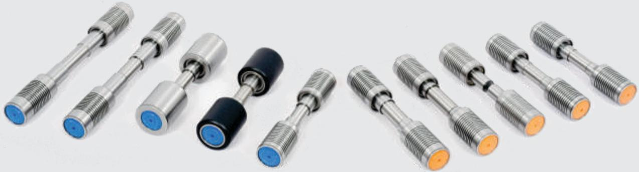
**T**op rollers are a pair of anti-friction, double row ball bearings having a common axle. Each top roller is manufactured such that the clearance between the hardened arbour and shell is perfectly matched with appropriately sized double row steel balls. The top rollers made for ring frames and speed frames are injected with just the right amount of a special grease – TRG 5. The ends are fitted with a uniquely designed seal to prevent leaks while in operation.
