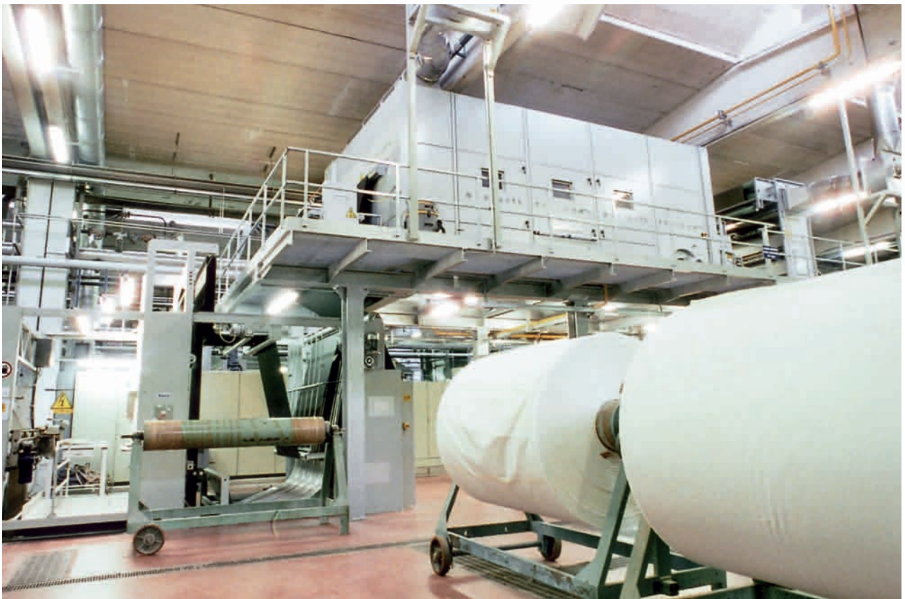
► Continuous dyeing range for the drying and thermosoling process ► 连续染色组合用于烘干与热熔工艺
