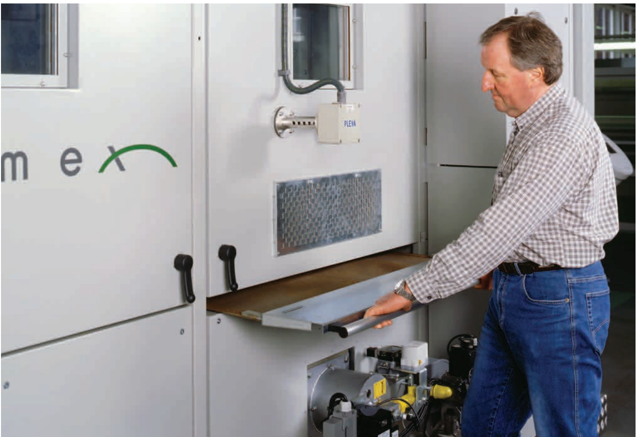
► Maintenance The lint filters can be pulled from outside the machine for cleaning during production.
