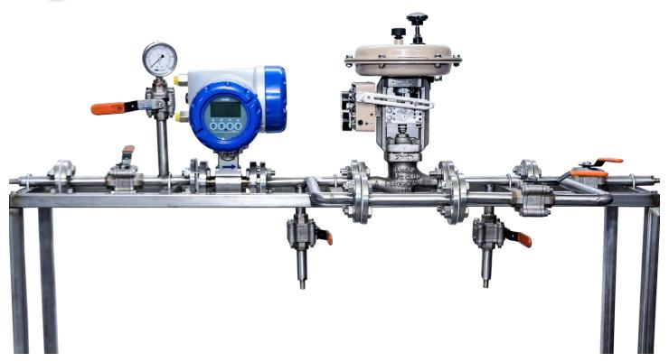
Usually used in denim yarn dyeing, the A.T.E. liquid indigo dosing system has precise flow control, ensuring accurate dosing of chemicals. The system includes both portable feeding units without speed control, as well as bulk feeding units which include speed control.
