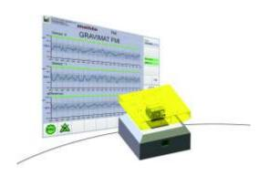
Mahlo's Gravimat measures the weight continuously, without contact, destruction-free and on moving products. The measurement is based on the attenuation of rays from a radioactive isotope through the substrate located in the measuring gap. This attenuation in intensity is an indication of the weight of the product.
