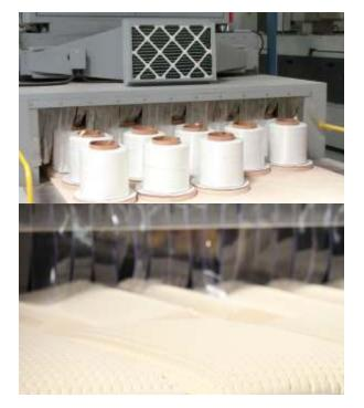
Stalam's RF equipment are the de-facto standard for the rapid and efficient drying of glass fibres, natural latex and SBR foams, medical PU foams, felts and other non-wovens. Stalam has also developed specific RF equipment to carry out innovative thermal processes such as the ribbonisation of glass fibres and the vulcanisation of latex foams.
