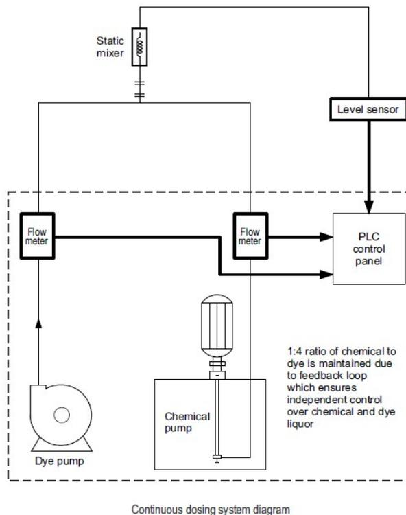
As shown in the diagram above, both the dye and chemical pumps are regulated through a feedback system that receives real time input from individual flow meters. Thus, the ratio is kept constant by controlling the speed of the chemical pump with help of a VFD (variable frequency drive) that is in sync with a dye pump. Even a small change in the flow of the dye pump is sensed and the chemical pump will act quickly to keep the ratio constant.
