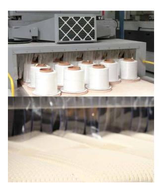
Stalam's RF equipment are the de-facto standard for the rapid and efficient drying of glass fibres, natural latex and SBR foams, medical PU foams, felts and other non-wovens. Stalam has also developed specific RF equipment to carry out innovative thermal processes such as the ribbonisation of glass fibres and the vulcanisation of latex foams.
