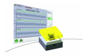
Mahlo's Gravimat measures the weight continuously, without contact, destruction-free and on moving products. The measurement is based on the attenuation of rays from a radioactive isotope through the substrate located in the measuring gap. This attenuation in intensity is an indication of the weight of the product.
