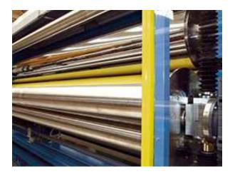
Designed in conjunction with Voith Paper - the renowned calender manufacturer, the NIPCO® HT (high technology) applies pressure where it is required, zone controlled and individually adjusted according to the material demands.
