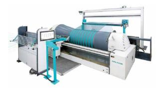
Warp preparation is important process to achieve the good quality fabrics and higher percentage of the fresh fabrics. KARL MAYER have various tension control solutions for fine yarns to coarser counts to have uniform tensioncontrolled warp beams across the length and width. This helps to achieve the required parameters of the warp beams with various applications.
