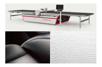
Morgan's Ply 1 is a high speed single layer cutting solution for custom production for apparel, home textiles and technical textiles. Ply1 offers high flexibility for customisation, fast production of small and irregular lots, and high performance.
