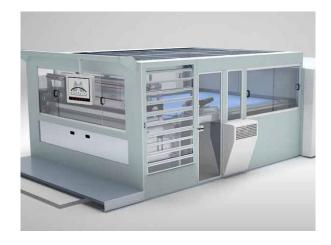
The patented modular Montex Allround offers a great deal of flexibility in coating and finishing. The Allround is a quick- change device that allows the necessary auxiliary modules to be docked to a basic module, thus enabling users to react quickly to new requirements.
