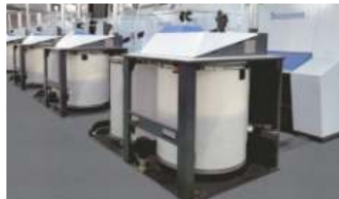
CCL: Linear can changer for 1,000 mm
