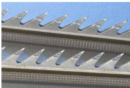
The TCC doffer wires are a standard design, the one below is of TCC scale-free quality.
