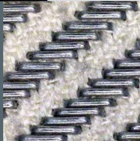
An exact geometry of the setting pattern on the back of a flat tops clothing strip.
