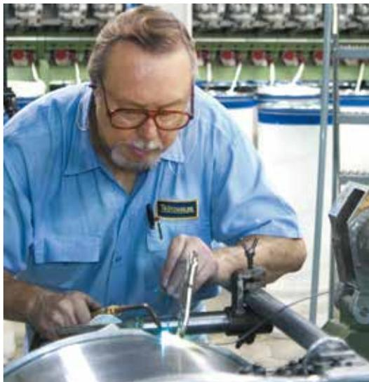
Fixing the wire end to a doffer roller
