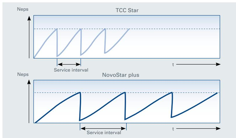
The wires in NovoStar plus quality lead to extended maintenance intervals and a considerably longer total service life.
