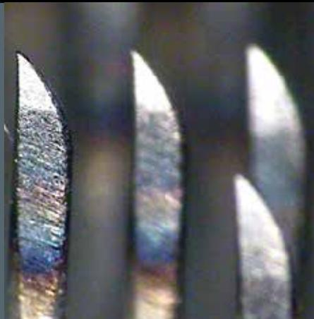
The bluish discolouration shows that the tips have been hardened after grinding.
