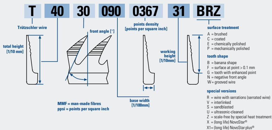
Trützschler Wire Identification Code – Every TCC metallic wire is clearly defined by the Trützschler Wire Identification Code. Here, the user can identify the tooth geometry, special versions or the surface quality immediately.
