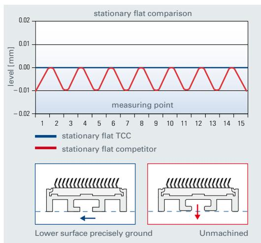
An absolutely even mounting is guaranteed by the precise machining of the wire carriers.
