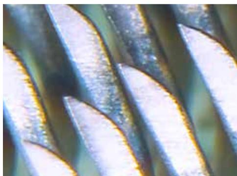
Precisely ground wire tips of flat tops before hardening
