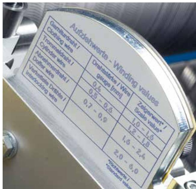
The winding tensions for all common wires are directly indicated on the T-Winder.
