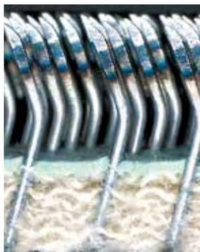
The cross section shows the embedding of the hooks in the foundation.
