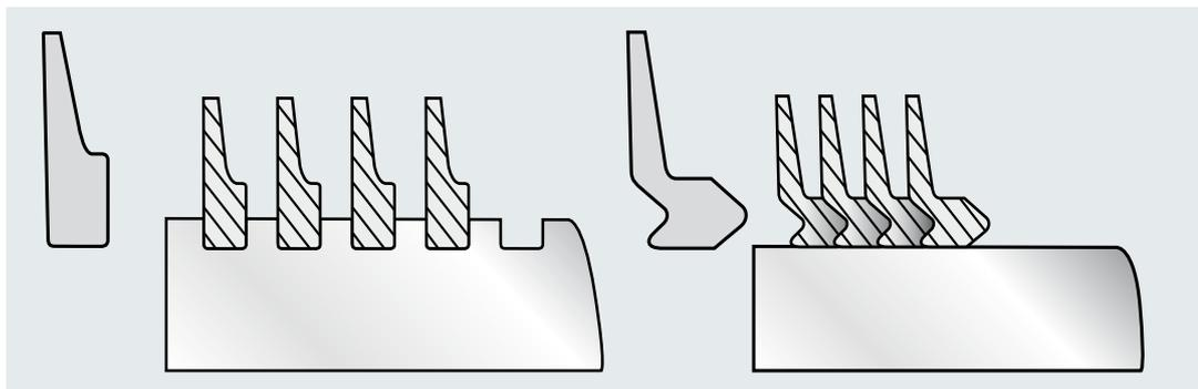
Lickerin wires can be mounted in grooves or interlinked
