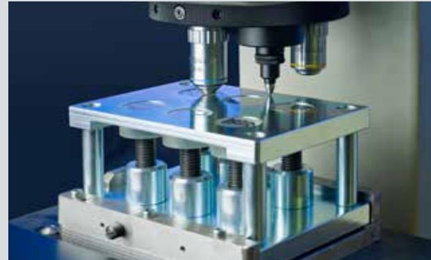
Part of the quality management system: wire samples are subjected to a hardness test.
