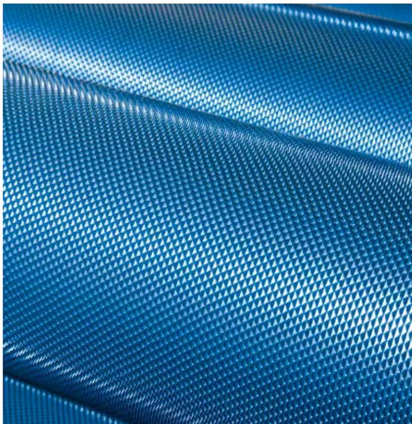
The photograph shows take-off rollers with special, electrolytically treated wires. These special wires need an extremely high-grade surface. Otherwise, even the adherence of single fibres may quickly result in lap formation.
