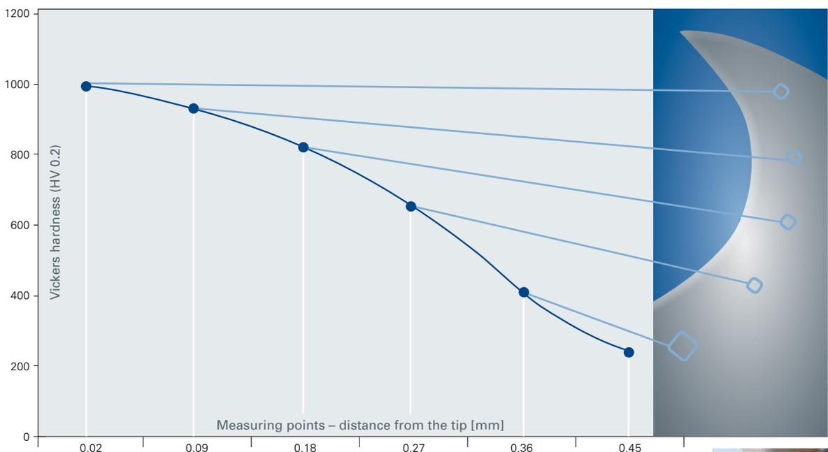
Result of a hardness test with typical hardness curve
