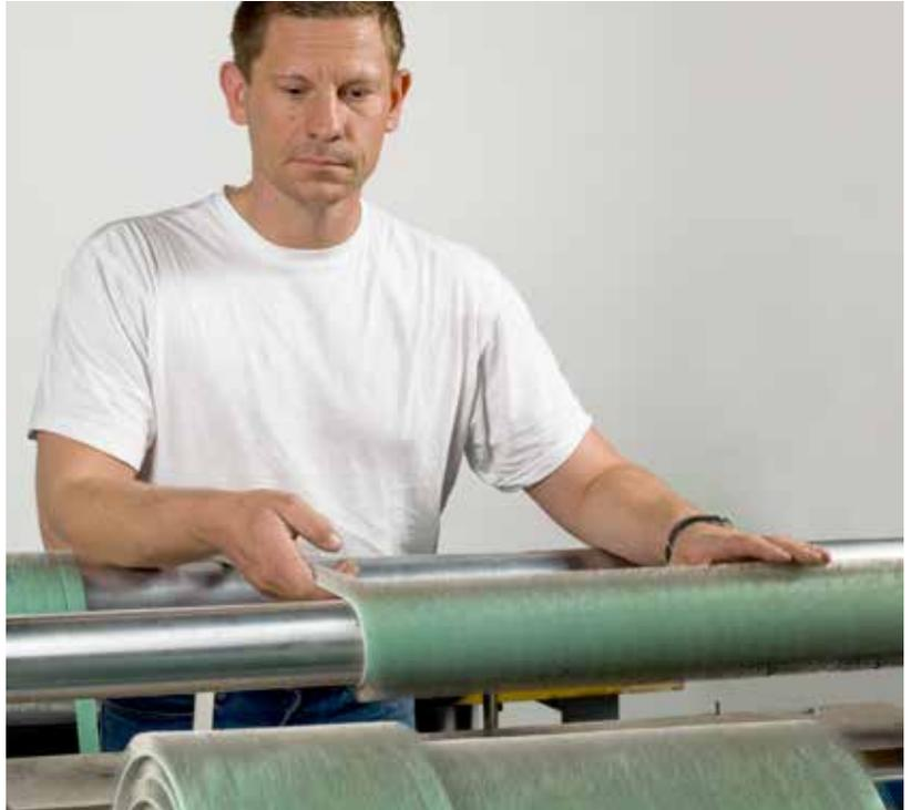
The flexible fillets, too, must be mounted very carefully on the roll body.
