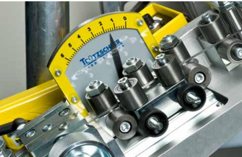
The T-Winder shows the actual winding tension.
