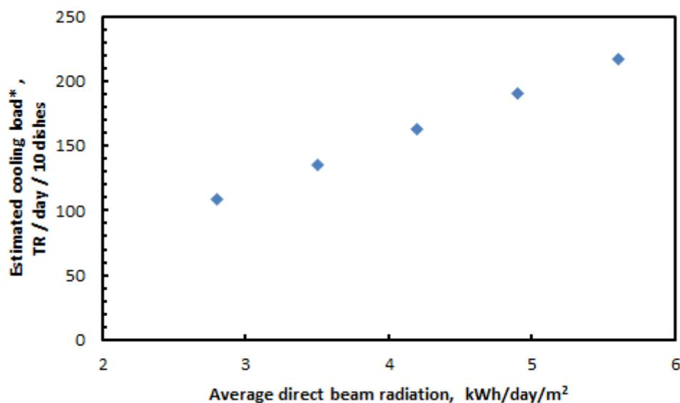
\* The cooling load calculated for 10 dish steam supply systems due to present limitation on commercially available VAM capacity
