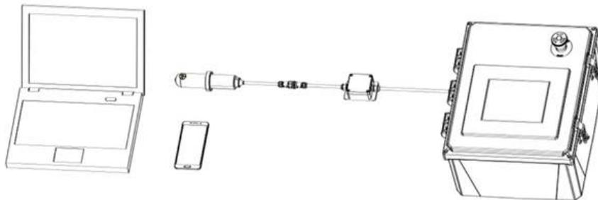
Figure 5. Bluetooth connection to ST-730 series probe
