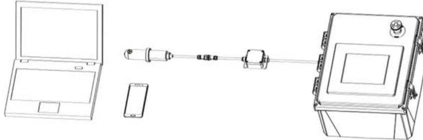
Figure 4. Bluetooth connection to ST-588 sensor
