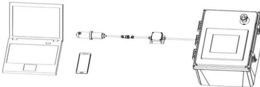
Figure 5. Bluetooth connection to ST-500 series probe
