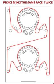
With two superimposed raising drums the machine has the possibility to process both faces of the fabric of twice the same face in one passage only. Moreover with the drums rotating in both directions it is possible to have a wide range of finishing effects.
