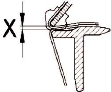
The vertical distance between the nose bar and the cradle at the nip point (distance 'X' in the figure above) determines the intensity with which the fibres being spun are controlled and guided between the top and bottom aprons in roving frames as well as in ring frames. To achieve optimum drafting conditions, the opening 'X' can be adjusted using distance clips to achieve best quality of yarn (in ring frames) and roving (in roving frames).
