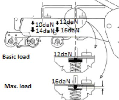
Two different loads are possible for the middle and rear top rollers. The load on the middle and rear top roller can be increased with a 4 mm allen key, by rotating 90° (approx) clockwise, from the current basic load position to increased load position. To return back to the
