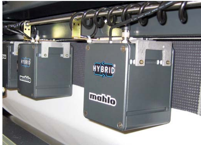
Automatic detection of change of fabric by Hybrid scanning®
