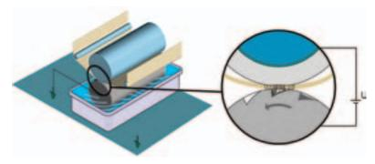
The Eltex electrostatic printing assist, ESA for short, is based on the principle of the plate-type capacitor. This means that a homogeneous electric field is generated between two plates, in which a dielectric is pulled to one side. The electrostatic printing assist applies this principle in the nip – at precisely the point where the ink is to be transferred onto the web.
