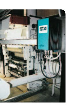
**The GNH61-System** is designed for installation in any gravure printing press. The work involved includes installing the charging and discharging bars, installing and connecting the generators, installing the remote control and wiring the system. Typically, a packaging gravure printing press with six or eight printing units can be fully ESA-equipped and ready for operation within one weekend.
