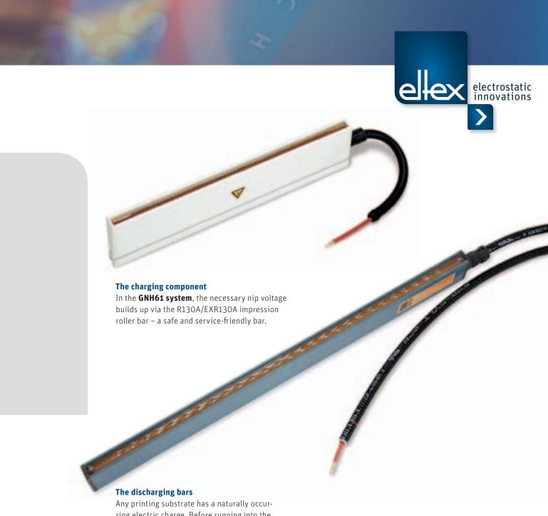
Any printing substrate has a naturally occurring electric charge. Before running into the nip, the web must first be discharged this is accomplished by the discharge bar R50/EXR50. The web is then charged up at the outlet; another discharge bar neutralizes the charges at this point. This means that two discharge bars are needed for each printing unit.
