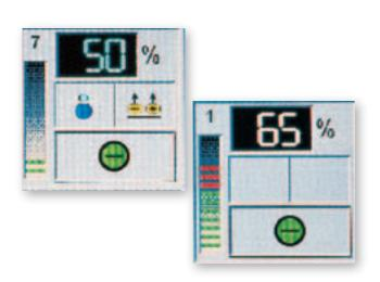
For example, when running the GNH61 system in paper operation, a status bar on the remote control indicates the level of pollution on the impression roller bar. As soil accumulates on the bar, the ESA system automatically increases the required voltage.
