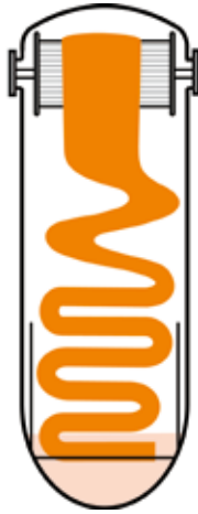
Medium Batch ECO-8: Single rope per tube
