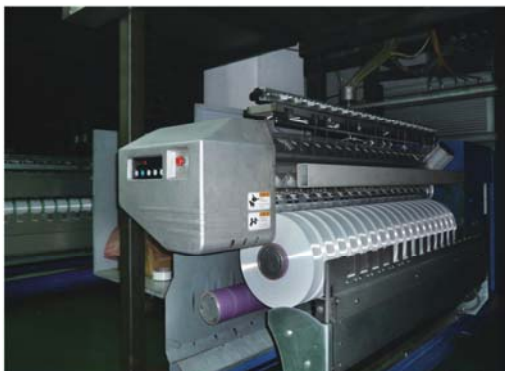
● 进口卷绕头的民用丝和工业丝改造技术。 Import winder's transformation technology for textural fiber and technical yarn
