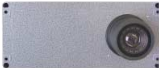
Traversing scanner with halogen lamp and spectrometer
