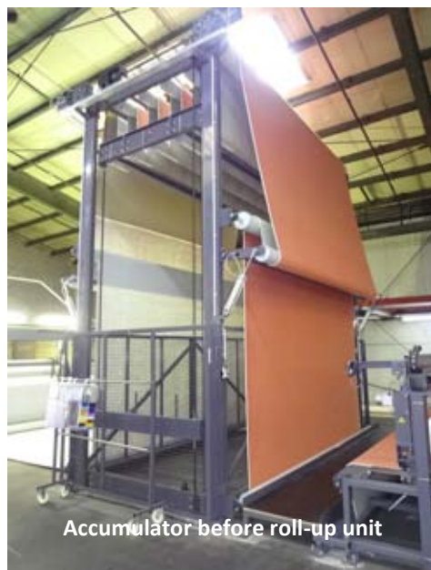
76 dpi print line at Maltzahn, Germany 420 cm width; 16 colors; 512 jets per color
