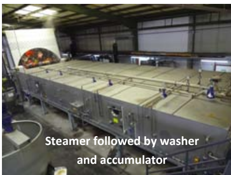
Unrolling, accumulator, pre-steaming, pre-washing, center guiding
