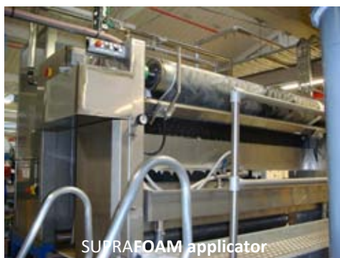
Carpet tile print line at Godfrey Hirst, Australia: 2,200 mm wide; 16 colors; 256 jets per color
