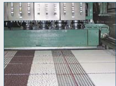
Positioned tiles during the printing process
