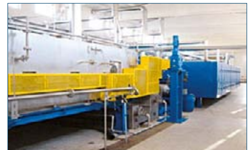
Horizontal steamer, washing unit and dryer
