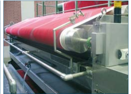
Foam application and impregnation
