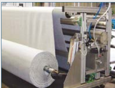
Unrolling unit with integrated pre-steamer, edge guiding and pull roller
