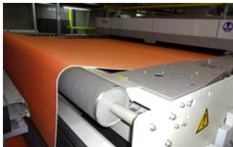
Exit of dryer with cooling zone
