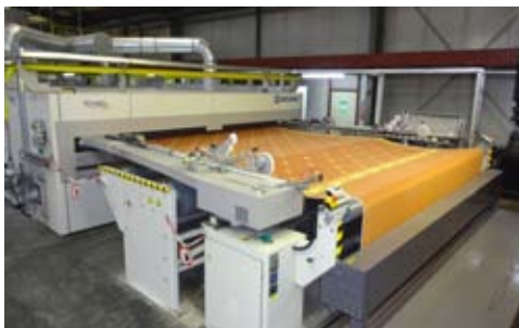
Stenter inlet to dryer
