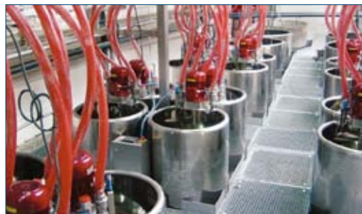
Color kitchen with automatic thickener and water dosing
