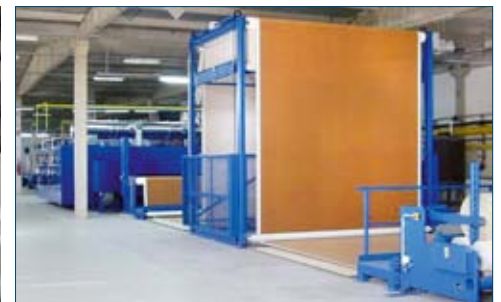
Accumulator, inspection zone, roll-up unit
