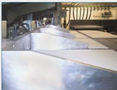
Carpet tile positioning device for a precise match of the print
