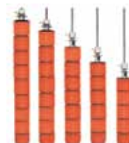
Flexible loading to maintain liquor ratio
