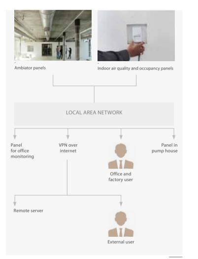
DIAGRAM OF THE MONITORING SYSTEM NETWORK
