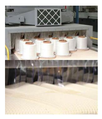
Stalam's RF equipment are the de-facto standard for the rapid and efficient drying of glass fibres, natural latex and SBR foams, medical PU foams, felts and other non-wovens. Stalam has also developed specific RF equipment to carry out innovative thermal processes such as the ribbonisation of glass fibres and the vulcanisation of latex foams.
