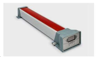
CEIA's TE/SLD is a highly sensitive bar metal detector. This device is ideal for protecting production lines against accidental damage caused by pieces of metal.
