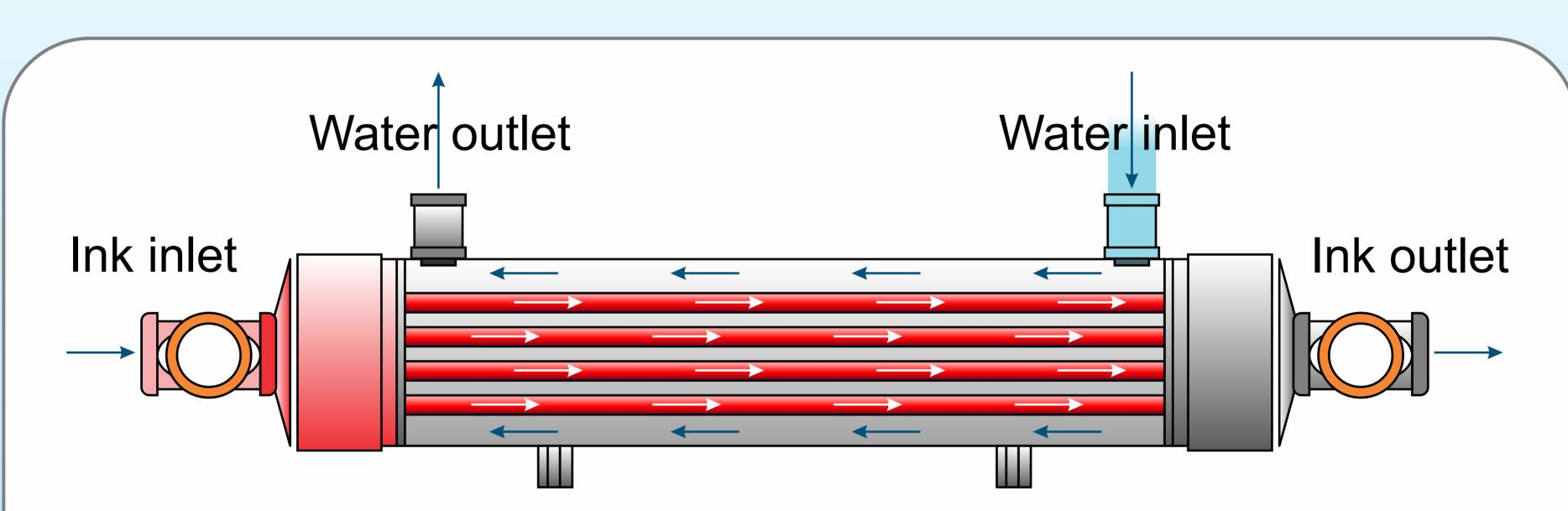
Valflow<sup>®</sup> Ink Temperature Stabiliser (ITS) cools the warm ink circulating in the press to a level that suits the process as well as the ambient conditions. This ensures consistency of printing and reduces top-up solvent and, in some cases, even ink consumption! The ITS has a leak-proof shell and tube heat exchanger design with chilled water as the media of heat transfer.
