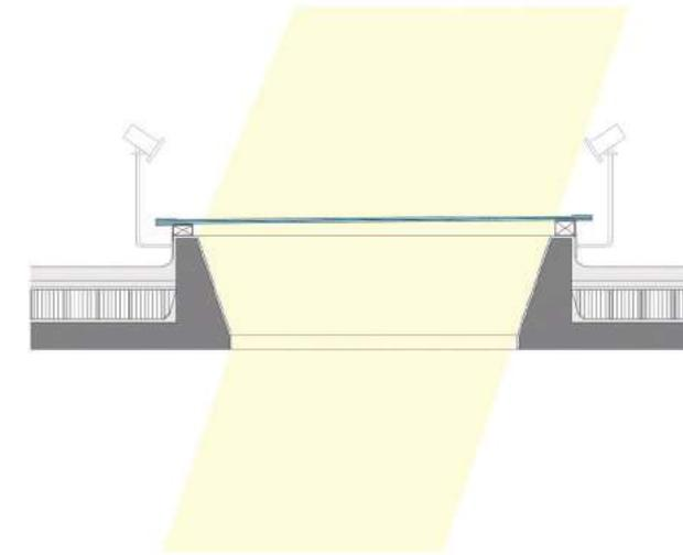
SECTION THROUGH ELLIPTICAL SKYLIGHT
