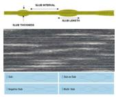
i.e., by changing the middle and back roller speeds as per required thickness and intervals. Today, the latest motion control technology with servo motors is used to produce slub yarn on ring frames.
