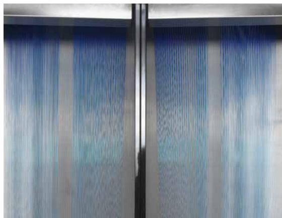
Quenching with 4 end per spinning position
