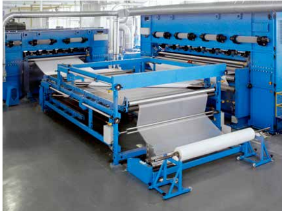
Needling machine installation for filter material
