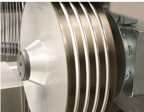
M40's cooling drum below the HPC texturing unit
