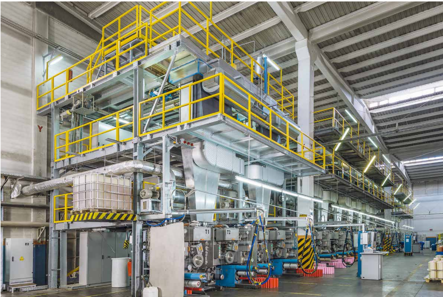
A M20/T20 mono- and tricolour BCF plant
