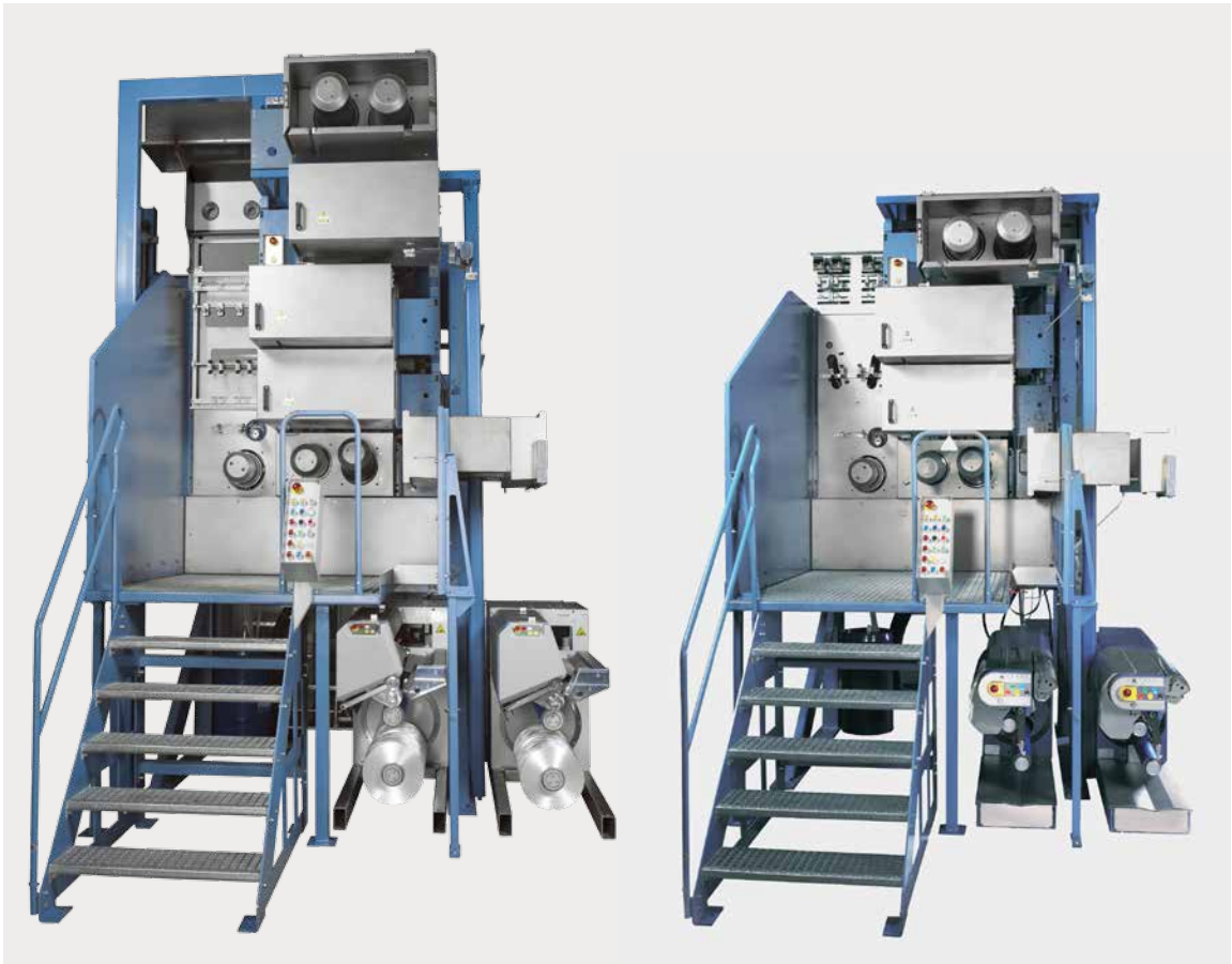
Draw panel with 5 duos for one spinning position
