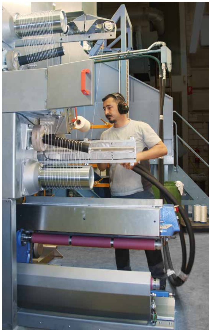
Stringing-up the BCF position
