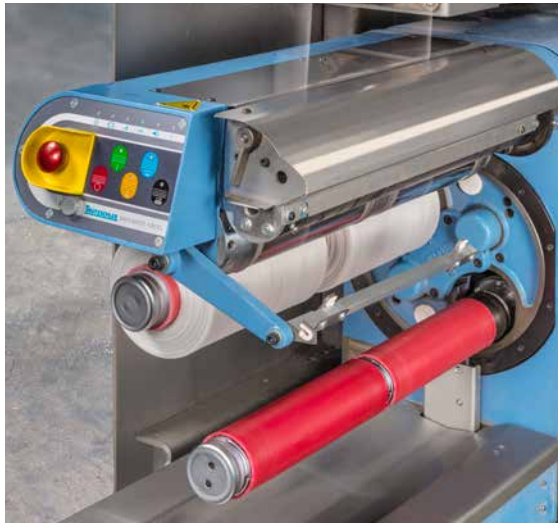
Winder and electrical upgrades
