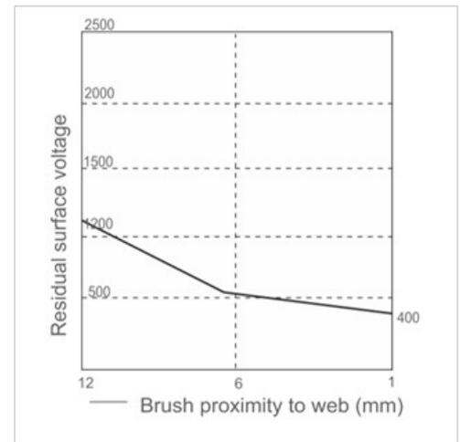
Effectiveness of Valstat® static discharge brush; in proximity to the web. Web speed 325m/min. Initial surface voltage - 10 kV
